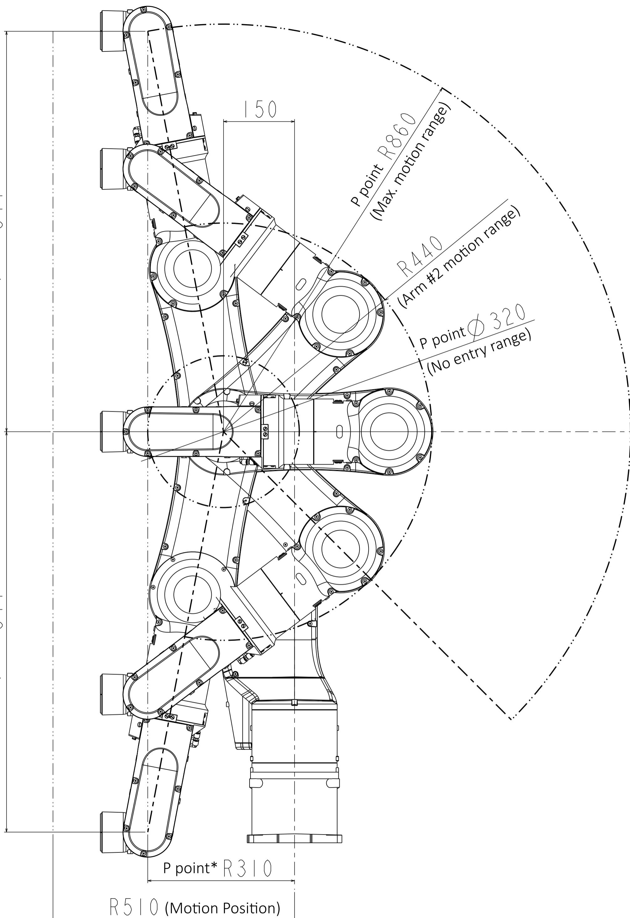
\* When the P point is 310mm apart from the center, upward and downward distance in CP motion will be the maximum.
